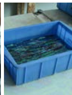
10. Soaking the sheets of Paua shell for hand punching - This is to prevent the shell from cracking
