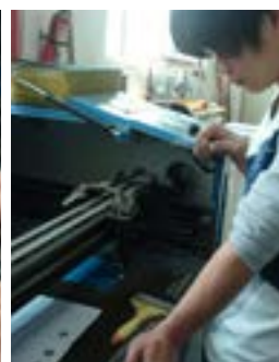
9. Making sure each piece of laser cut shell fits exactly into the metal part
