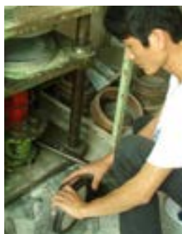
2. Opening the mould after casting.
