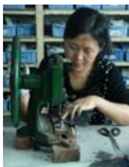
11. Hand punching the shell pieces that are too small to be laser cut.
